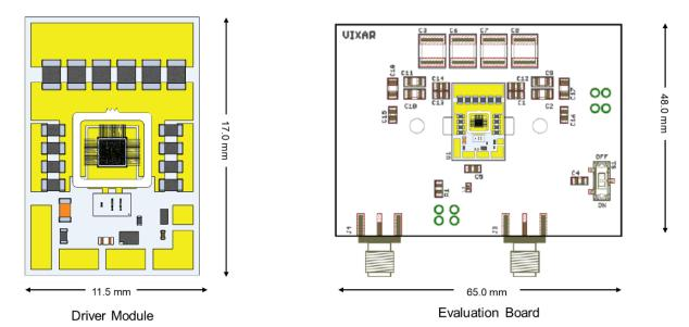
Figure 01: VCSEL driver circuit (left) and evaluation module (right).
