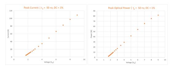
Figure 05: Measurement results for peak current (left) and peak optical power (right) as a function of supply voltage.
