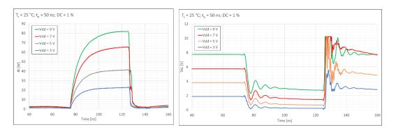
Figure 04: Measurement results for optical pulse power (left) and TAL voltage (right).
