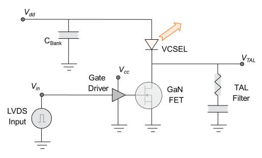
Figure 02: Circuit illustration of the driver module.
