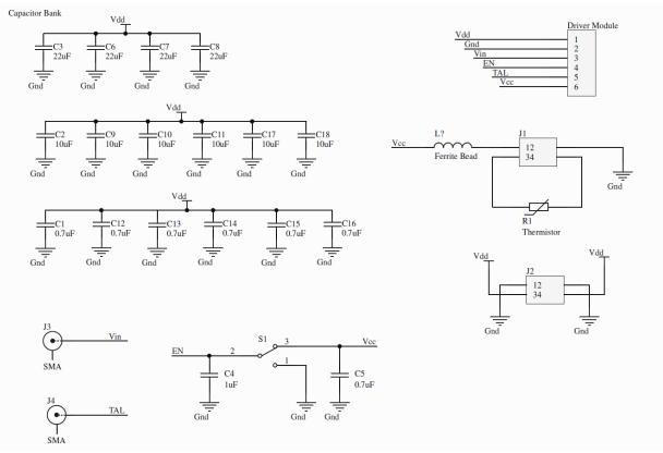
Figure 08: Schematic of the VCSEL evaluation board.
