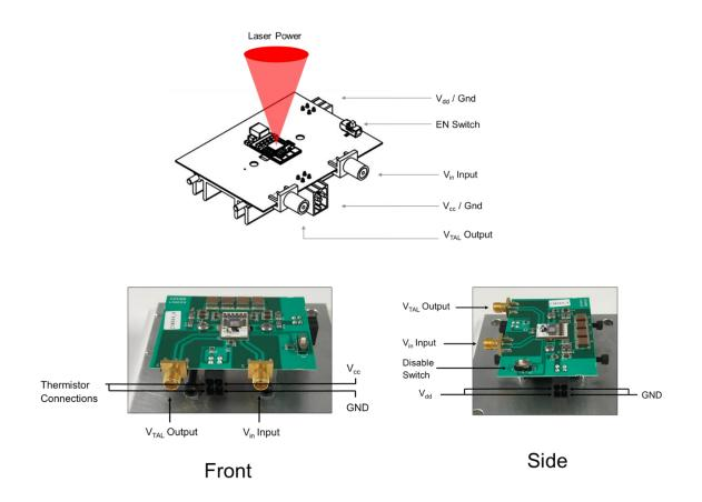
Figure 03: Connections for VCSEL evaluation board.
