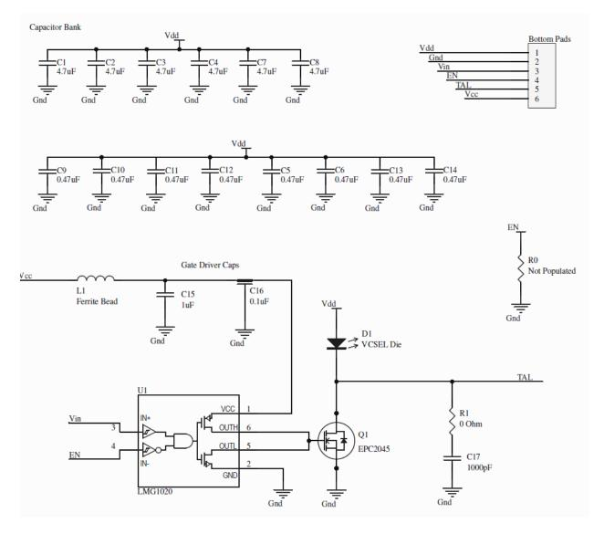
Figure 07: Schematic of the VCSEL driver module.
