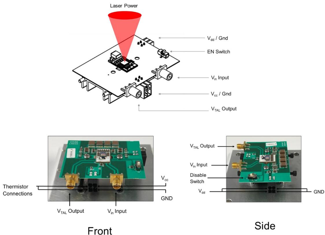
**Figure 03:** Connections for VCSEL evaluation board.
