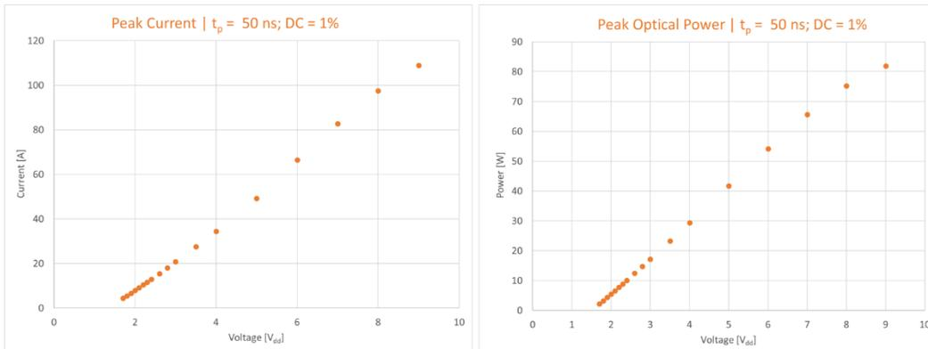
**Figure 05:** Measurement results for peak current (left) and peak optical power (right) as a function of supply voltage.
