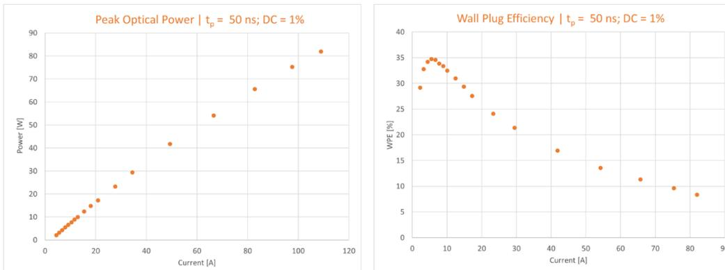
**Figure 06:** Measurement results for peak optical power (left) and driver module wall plug efficiency (right) as a function of peak current.
