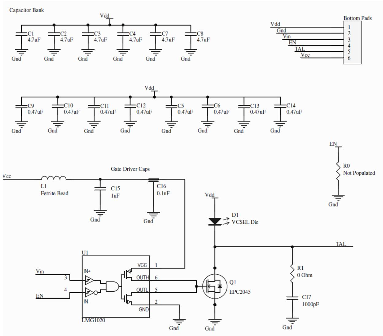
**Figure 07:** Schematic of the VCSEL driver module.
