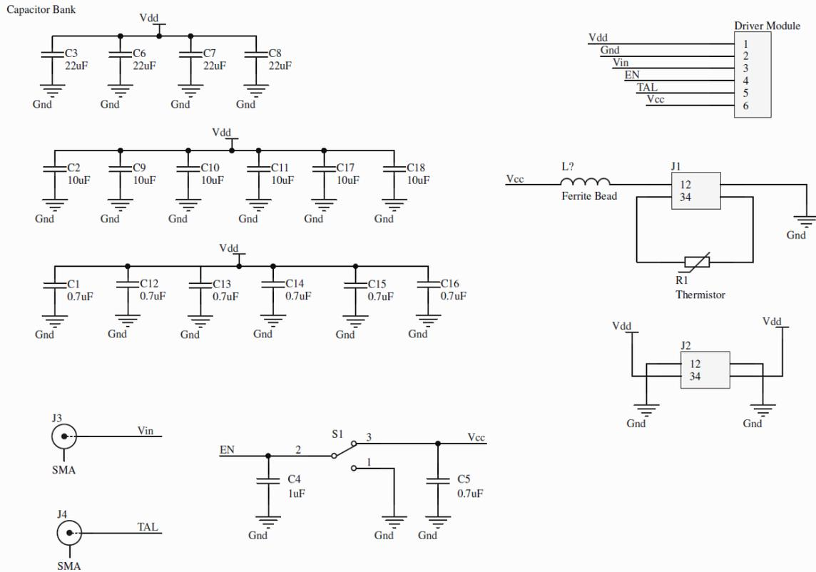
**Figure 08:** Schematic of the VCSEL evaluation board.
