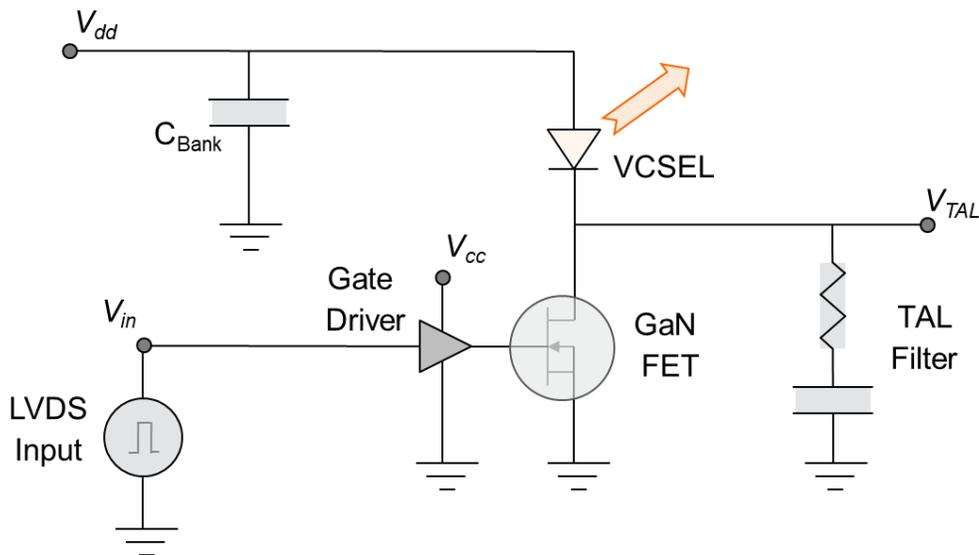
**Figure 02:** Circuit illustration of the driver module.
