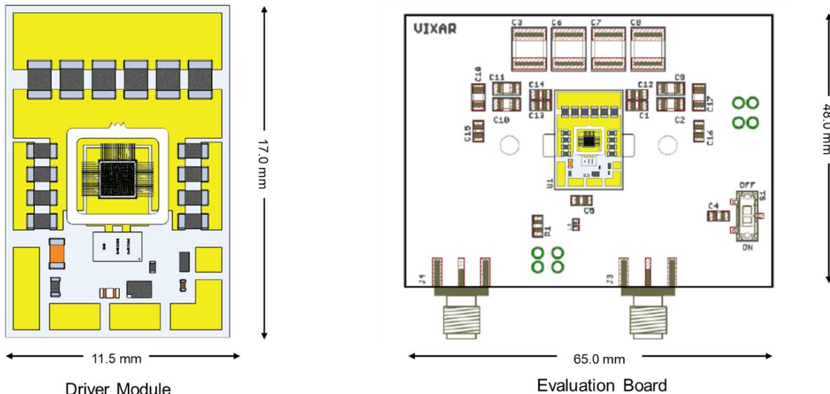
**Figure 01:** Vixar driver module (left) and evaluation mother board (right).
