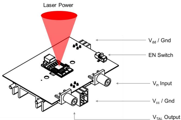
**Figure 03:** Connections for VCSEL evaluation board.
