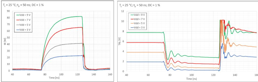
**Figure 04:** Measurement results for optical pulse power (left) and TAL voltage (right).
