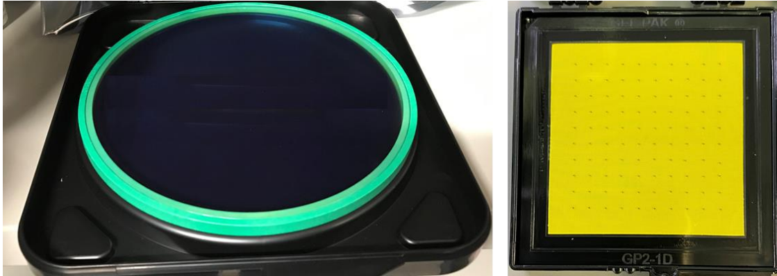
Figure 4: Plastic hoop ring with non-UV tape used for VCSEL die delivery (left). VCSEL die placed on Gel-Pak (right).
