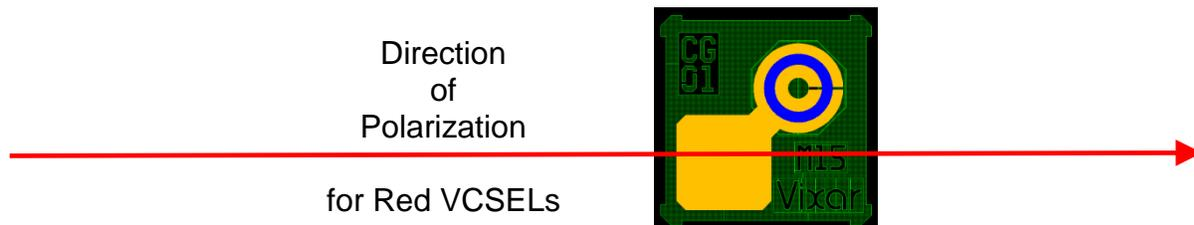
4. Vixar's 795 nm & 895 nm VCSELs also emit a linear polarized beam. Contact Vixar for details regarding the direction of polarization for these devices. Polarization of these devices can be impacted by die attach process (see Note 5) and encapsulants (see Note 8).
